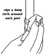
Integral solder type. These are worked in a very similar fashion except that the solder is already in place and as soon as sufficient heat has been applied, it will be drawn from its groove into the narrow gap between fitting and pipe.
