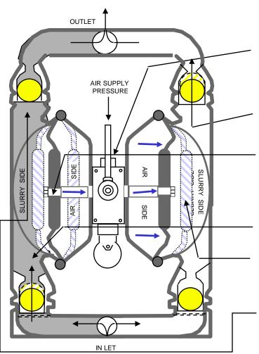
Patented, one-moving-part air valve directs air supply to back side of diaphragm
